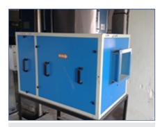
These modules consist of 5 and or 10 micron filters with a low static centrifugal fan along with motor mounted on common base frame and aluminium air diffuse at discharge.
